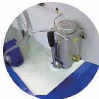
XYZ导轨集中润滑 Central lubrication for XYZ axis
