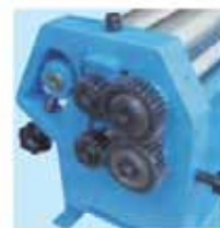
Hardened steel gearing
