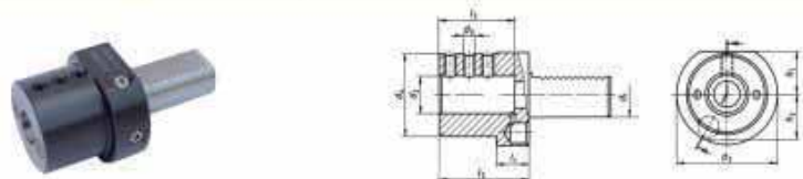
■ ZZ-003268 E2型圆柱孔刀夹 (铣、镗孔) TYPE E2 TOOL HOLDER for boring bars with cylindrical shank
