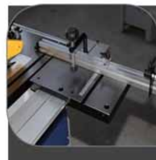
CAST IRON SLIDING CARRIAGE WITH FOUR WHEELS
